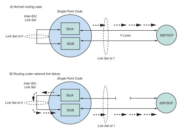
Figure 6. Transmit Routing to a Single Destination
